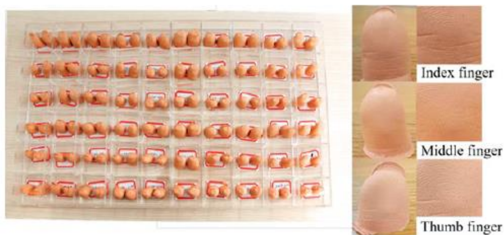
Figure 22. An array of high-precision fake fingers modeled from index, middle, and thumb fingers from 20 subjects 101
